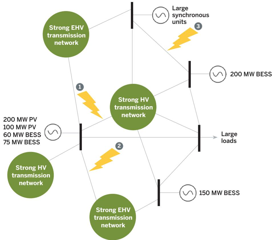
**A strong region within the ATC system used to test the stability of multiple GFM BESS in close proximity (left side of the figure). Key disturbances were simulated to test for stable behavior.**
