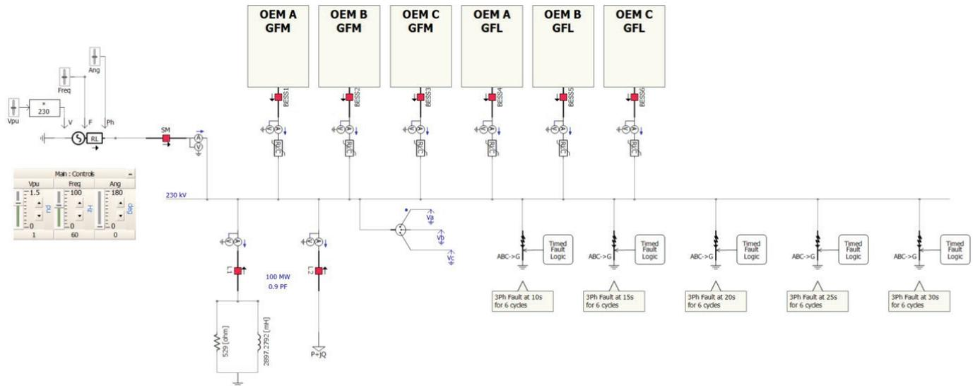
**Testbed for focused evaluation of manufacturer-supplied BESS models.**
