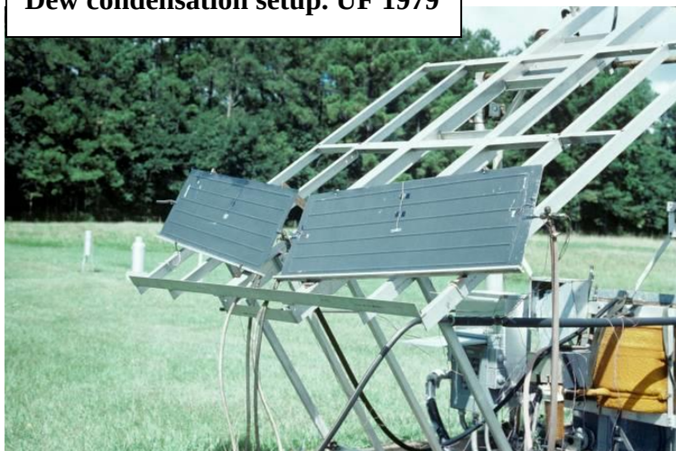
Dew condensation setup. UF 1979
