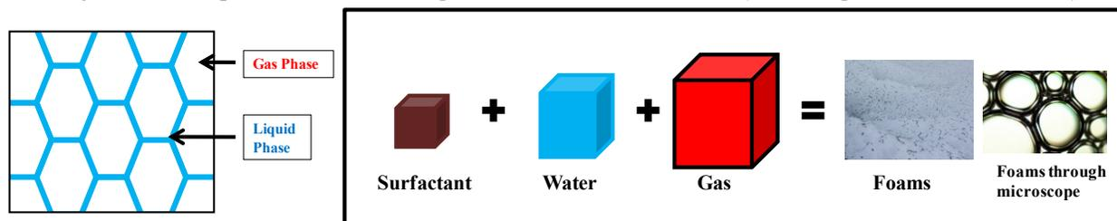
**Figure 2.2:** Structure and formation of foam in lakes
